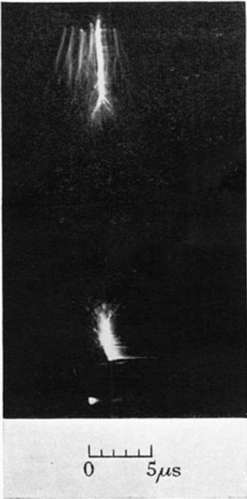
FIGURE 15. Time-resolved photograph of arrested breakdown in a 75 cm diameter sphere/rod gap at 900 kV crest voltage; gap spacing 65 cm; wave shape 0.50/2000 \mu s.
